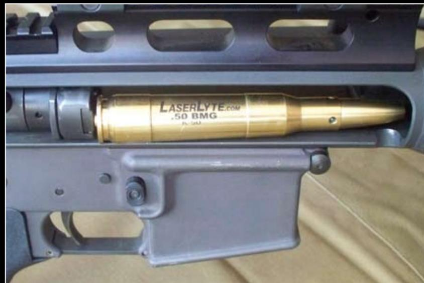
The easy way to cut cost while zeroing a .50 BMG is the LaserLyte Bore Tool. The green Kryptonite laser is easily visible even in bright sunlight.
