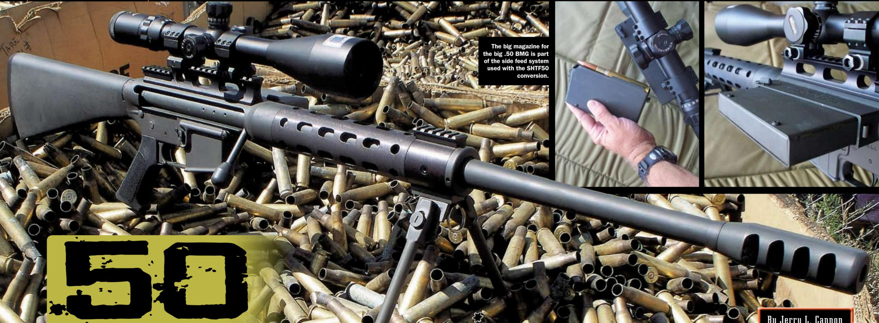
The big magazine for the big .50 BMG is part of the side feed system used with the SHTF50 conversion.
