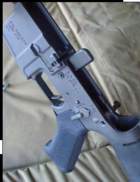
**Included with SHTF50 conversion is a heavy hammer, to ensure a solid firing-pin strike and ensure primer ignition.**
