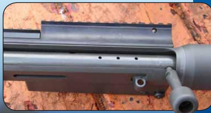
*On the SHTF-50, everything is big and built for use, from the hefty bolt to the long bolt handle for better leverage in working the action.*
